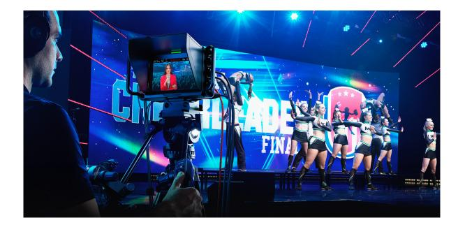
Again, a multi-camera combination of Studio Camera 4K Pro and ATEM Television Studio Pro 4K switcher is an ideal match for this application because SDI connectivity is necessary in venues where camera positions are likely to be located more than 10m from the switcher. Depending on cable quality, SDI can be used for lengths up to 100m with the added advantage the cables are more rugged, with BNC twist lock connectors to prevent them from being pulled out accidentally.
